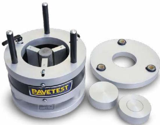
**B202** Gauge Point Fixing Jig + accessories for small specimens preparation
