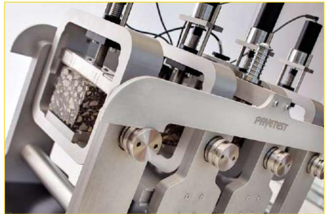
**B210-01** Servo-pneumatic four point apparatus, detail
