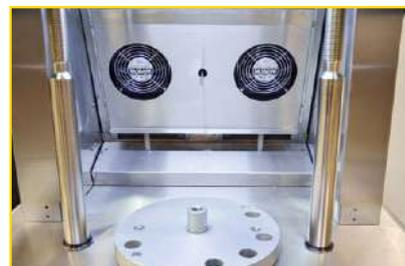
Recirculation fans ensuring uniform temperature in the chamber.
