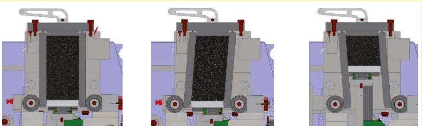
During the compaction process a lateral displacement is applied to the specimen along with a vertical load, which results in a shearing action that makes the compaction similar to the the field.
