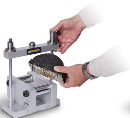
Asphalt specimen positioning
