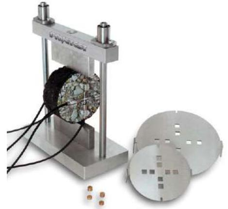
**B253 KIT** Indirect Tensile modulus, creep compliance and strength using on-specimen transducers
