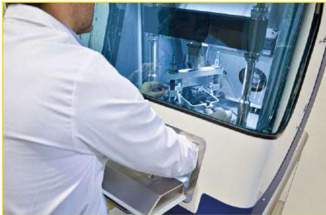
A small window offering access to the test space with minimal disruption to the chamber temperature.
