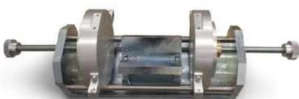
**B282-08** TSRST specimen gluing jig (needed accessory)
