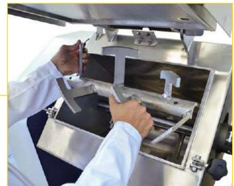
Detail of the detachable mixing shaft with helical blades
