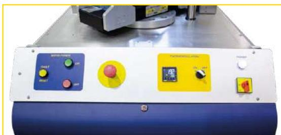
Thermoregulation display to monitor the temperature in real time.
