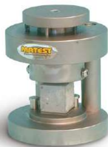
E170 COMPRESSION TEST ON MORTAR SPECIMENS
