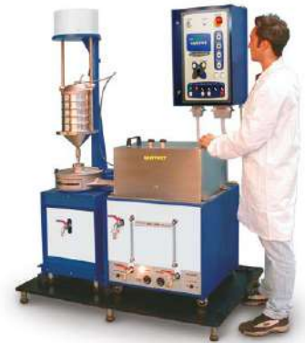
B008 AUTOMATIC BINDER EXTRACTION UNIT
