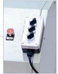
Standard model, low clamping pressure only (3 buttons)
