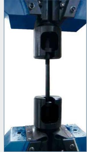
Tension on threaded and shouldered head samples
