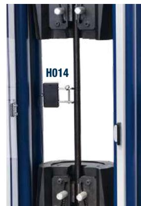
**ELECTRONIC EXTENSOMETER FOR TENSILE DEFORMATION STRENGTH TESTS UNTIL BREAKAGE**
