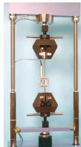
S205-05N + accessories for tensile test
