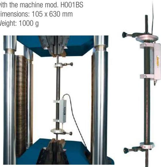
**ELECTRONIC EXTENSOMETER FOR TENSILE DEFORMATION STRENGTH TESTS UNTIL BREAKAGE**
